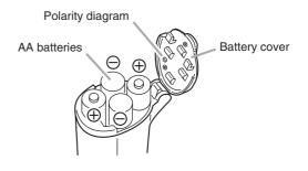
Step 3. Press the battery cover down and slide it in the direction of the arrow until it clicks to lock.
