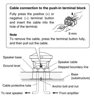
Step 1. Connect the speaker cables that have been run through the cable protective tube to the push-in terminals inside the speaker base.
