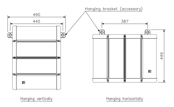
Note: Every speaker module must be aimed horizontally or down to keep the weather resistant capability.
